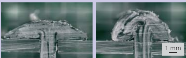
Cross section images of two formed fiber-reinforced plastic webs
