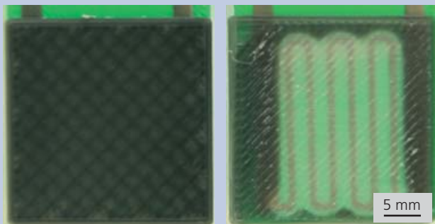
FFF component with integrated heating elements
