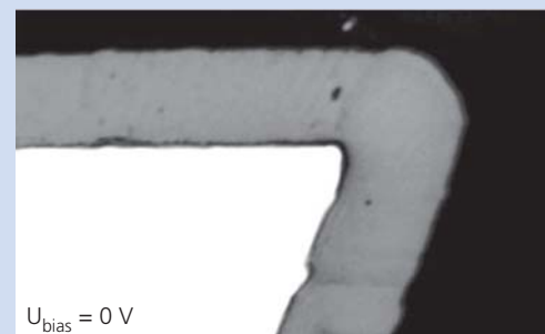
Transverse microsection of a monolayer coating, deposited without bias potential (top) and a multilayer hard coating, deposited with high bias potential (bottom)
